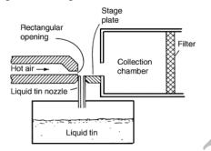
Figure 1: Cross – jet gas atomization scheme. [3]
