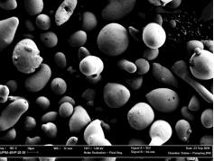
Figure 4: Scanning electron micrographs of gas atomized tin powder.
