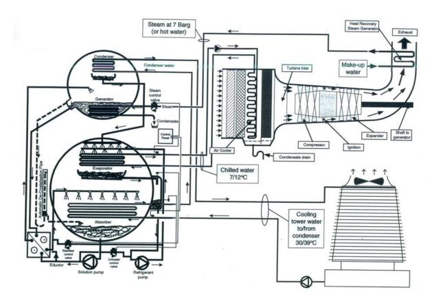
Figure 2. Inlet air cooling system
