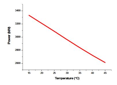
Figure 4. Graph between the Power Output of the Gas turbine and Temperature
