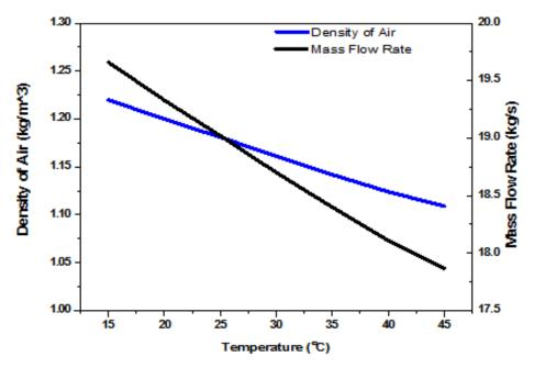
Figure 3. Graph between Density, Mass Flow Rate of Air and Temperature
