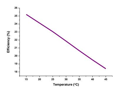
Figure 6. Graph between the Efficiency of Gas turbine and Temperature
